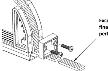
Excess strap length may be cut after final adjustments have been performed.
