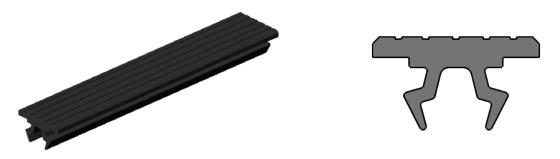
To insert channel cushion, center over strut or extrusion and press in. Lubricate with a soap & water solution underside of channel cushion to assist in assembly.
