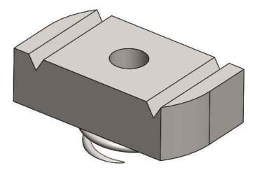
Channel Nuts hold brackets to our PAC Trac and Dual Trac extrusions. These inserts lock in the tracks when the screw is tightened. Loosen the screws and the Channel Nuts can be moved or removed.
