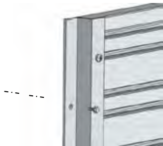
SCREW MOUNTING WITH Z-MOUNT
