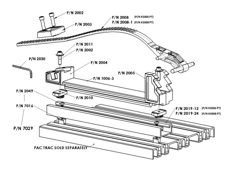
Place Trac Lok inserts **P/N 7016** into channel on **PAC TRAC** in desired location and attach Unistrut with screws. Tighten to a <u>maximum</u> 15 in-lbs
