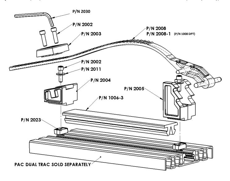
Attach modules to Unistrut with P/N 2023 channel nuts.
