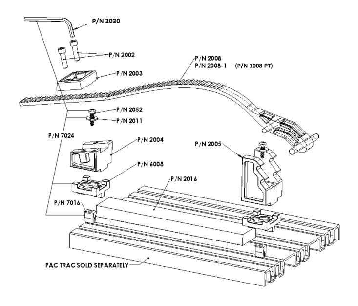
Place Trac Lok inserts **P/N 7016** into channel on **PAC TRAC** in desired location and attach modules with screws. Tighten to a <u>maximum</u> 15 in-lbs
