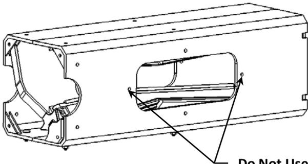
**CAUTION:** Never use the two plugged center holes around the window for mounting. Air cylinders may be damaged by fasteners.
